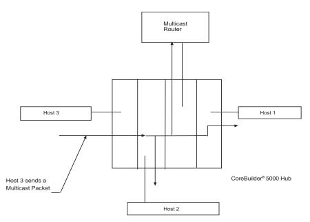
Figure 5-1 shows a typical packet path before snooping occurs.
